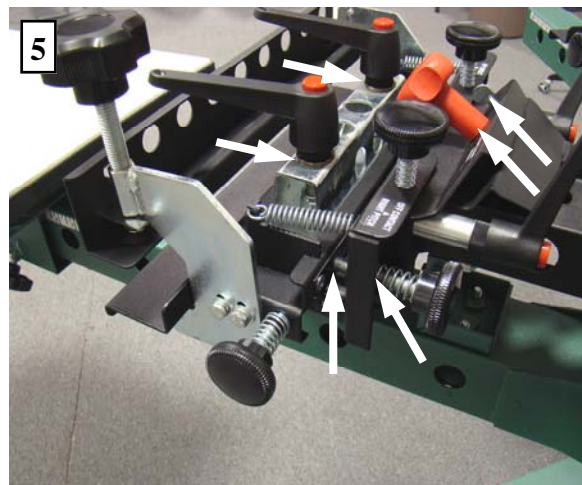
Micro Adj. Locking Levers Micro Adj. Knobs & Wear Plates (both sides) Front / rear Pitch Knob, Locking Screw Thread Lubricants
